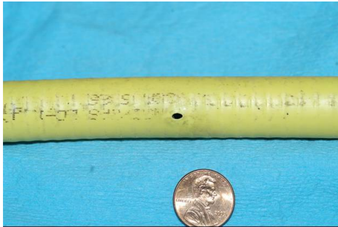
Figure 7: Photo of perforated CSST without pyrolysis
