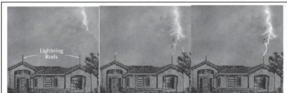
Graphic shows (1) downward leader descending from cloud (left picture); (2) upward streamers emerging from lightning rods and tree (middle picture); and (3) leader-streamer connection (right picture).
