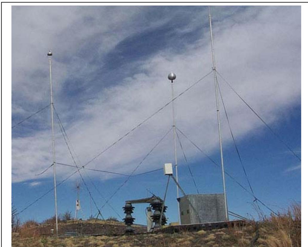
This picture shows of one of the New Mexico test sites where several types of ESE (French and Australian air terminals) and conventional air terminals had been exposed to lightning for several years to gauge their effectiveness under natural lightning conditions.
