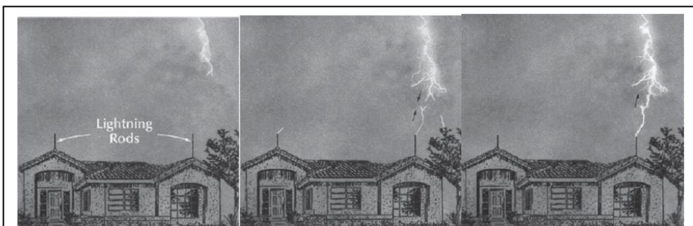
Graphic shows (1) downward leader descending from cloud (left picture); (2) upward streamers emerging from lightning rods and tree (middle picture); and (3) leader-streamer connection (right picture).
